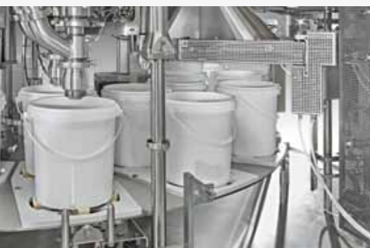
2-lane, weigh-controlled filling station
