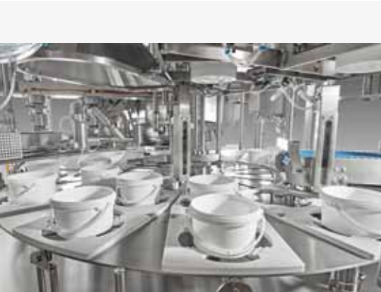
View into the 2-lane rotary table; it is designed for round and rectangular buckets
