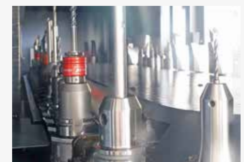
View into the tool changer of the universal lathe for 60 tools.
