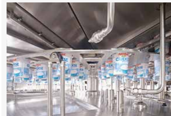
In the middle of the picture one of the spraying nozzles of the fully-automatic interior cleaning for foaming and rinsing the rotary table; optional supplementary equipment: complete interior cleaning with heated laminar air
