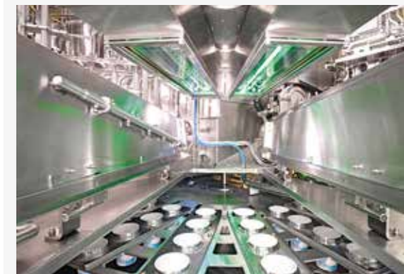
The high-performance radiators of the 2-phase pulsed light high-performance UV(C) sterilisation procedure in the hygiene tunnel of the UC rotary-type cup filler
