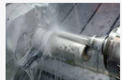
Machining of the sleeve on the universal lathe type CLX 450 TC.
