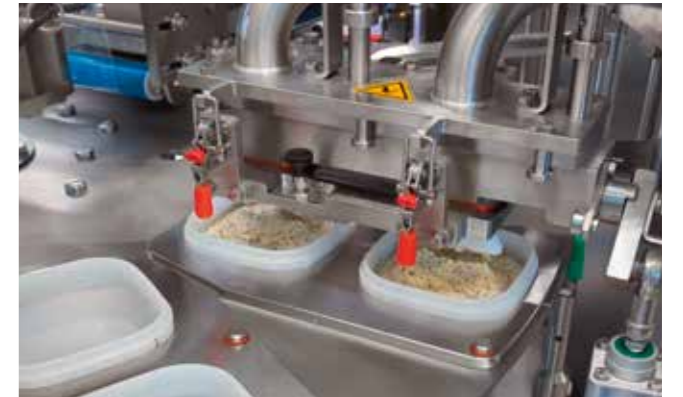
Filling station with integrated weigher with automatic weight readjustment
