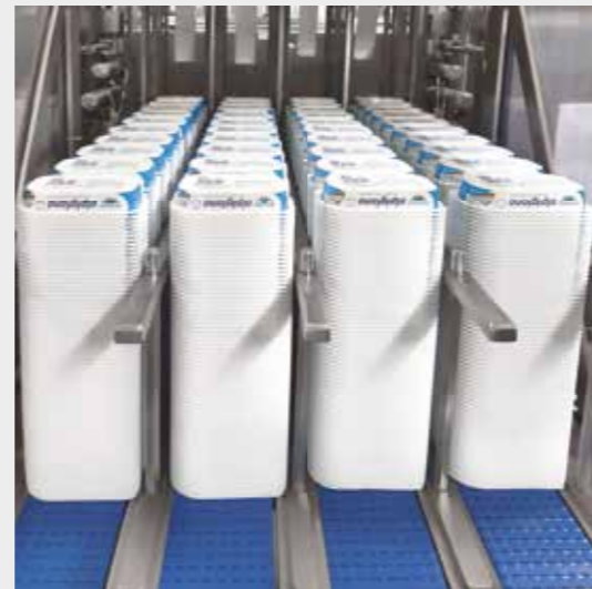
Cup loading station; the cups are stacked upside down
