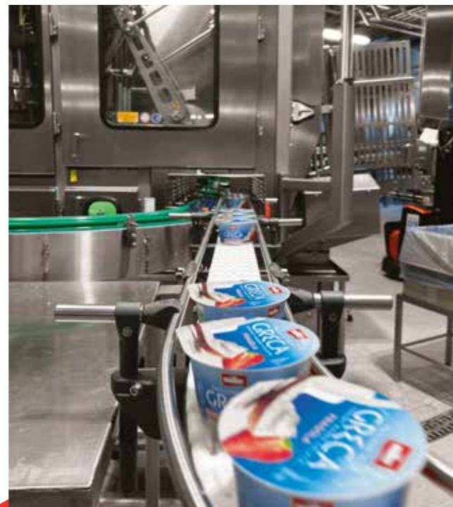
Photos taken during the commissioning of the 4-lane (UC) rotary-type cup filling machine
