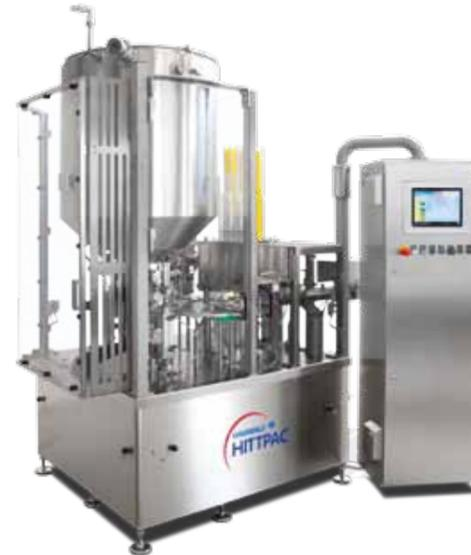
Frumarco enquired a flexible, solid and high-performance machine for handling cups of different filling volumes from 15 grs - 80 grs which should also be space-saving due to the limited space available. The model GRUNWALD-HITTPAC AKH-019 could meet all these requirements.
