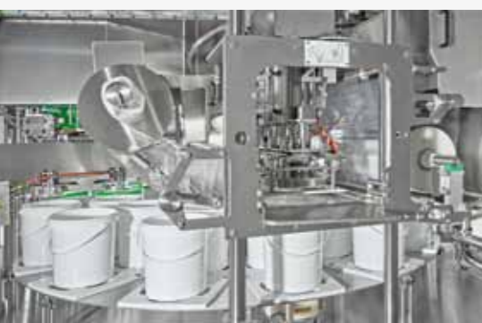
Cutting/sealing station for film from the reel with easy and quick change of the cutting die
