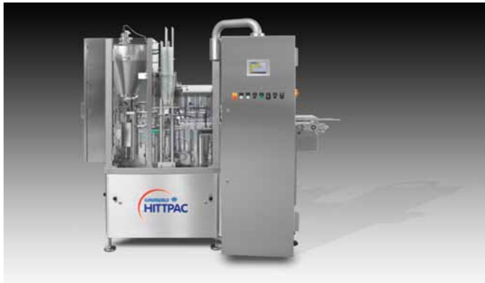
The cup filler GRUNWALD-HITPAC AKH-019S/2-lane supplied in 2012 for filling dips and sauces in round plastic cups Production speed: up to 5,000 cups/h
