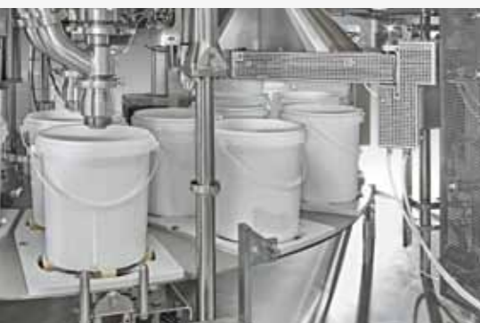
2-lane, weigh-controlled filling station
