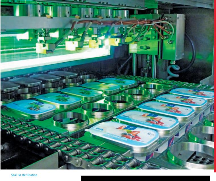
using UV(C) light highpressure radiators. The picture also shows a cup transport with double advance feed which gives quick format changes
