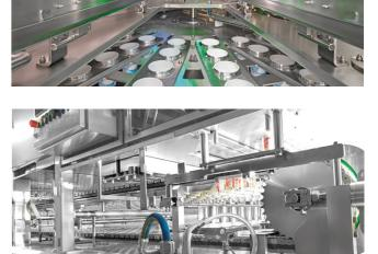
Insight into high-performance filling machines: Rotary-type and linear cup filling machines in ultraclean design and with packaging material sterilisation  $\geq$  LOG 4
