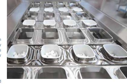
View into a 4-lane cup filling and closing machine GRUNWALD-FOODLINER 6.000 in double-step
