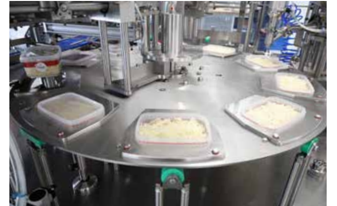
View on the rotary table – while filling rectangular cups
