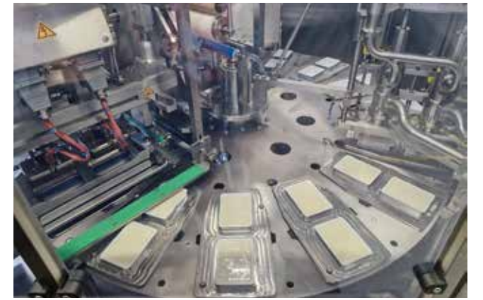
View into the rotary-type filling machine while filling silken tofu in a 400 g tray
