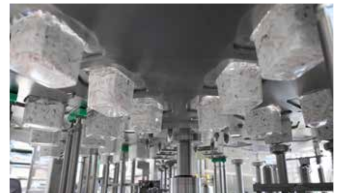
The view into the 3-lane GRUNWALD-ROTARY 12.000 shows the rotary table while filling meat salad
