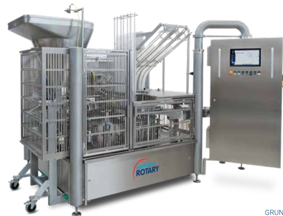
The view into the 3-lane GRUNWALD-ROTARY 12.000 shows the rotary table while filling meat salad
