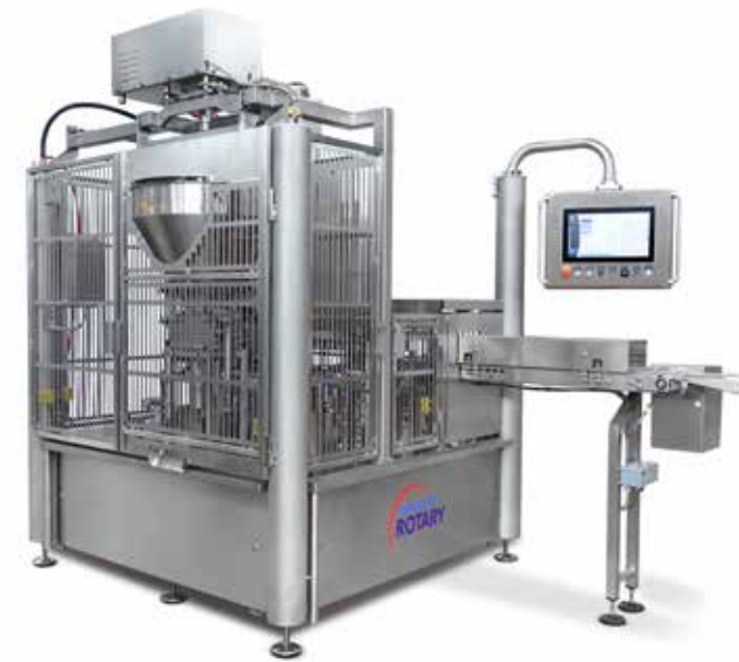
One of the GRUNWALD-ROTARY 6.000 machines at Petri Feinkost: precise filling of vegan cream cheese at 42 cycles per minute
