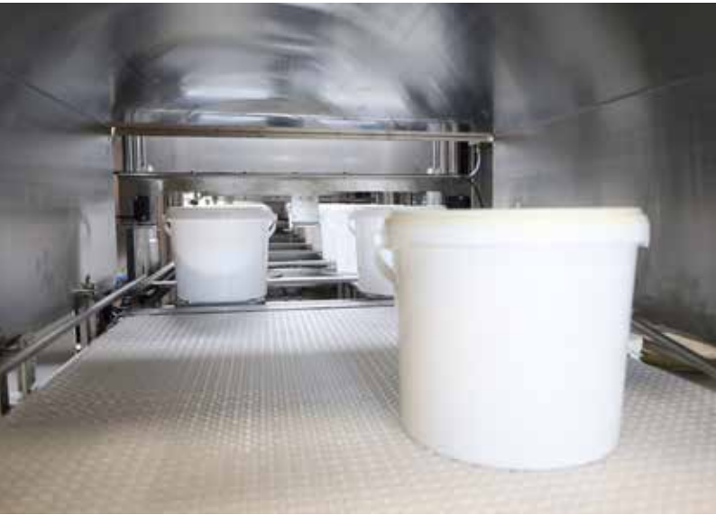
Photos above: A look inside the bucket filling line
